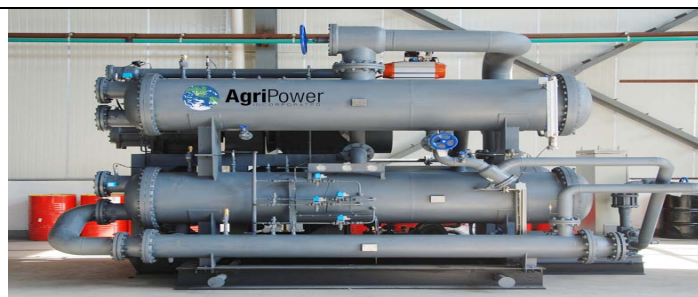
Waste Heat Electric Generator
